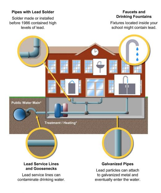
\*Regardless of whether your school's drinking water is supplied by a municipal water system or its own well, the water will enter the building through a service line(s). Once inside the building, water may undergo treatment for impurities and heating before being distributed to various fixtures in the building via a network of pipes.
